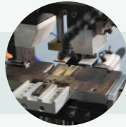
Nose bridge bending
